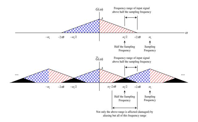
So, it is clear that not only the range of the input signal  $[\omega_s/2, 2\pi B]$  gets affected by aliasing, but all the range from  $[\omega_s-2\pi B, 2\pi B]$  is affected by aliasing.
