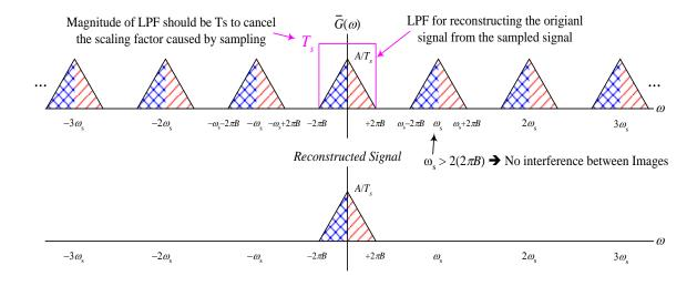
If the signal was sampled at a sampling rate lower that 2 times the bandwidth of the signal (called the **<u>NYQUIST SAMPLING RATE</u>**), the different spectral components of the sampled signal (called IMAGES) will interfere with each other and reconstructing the original signal will be impossible. This is illustrated in the following figure. The dark parts in the figure represent parts of the sampled signal and reconstructed signal that have been damaged.
