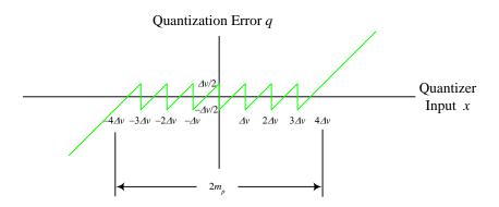
It is seen from this figure that the quantization error of any sample is restricted between  $-\Delta v/2$  and  $\Delta v/2$  except when the input signal exceeds the range of quantization of  $-m_p$  to  $m_{p.}$
