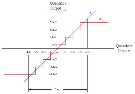
Now let us define the quantization error represented by the difference between the input sample and the corresponding output sample to be q, or
