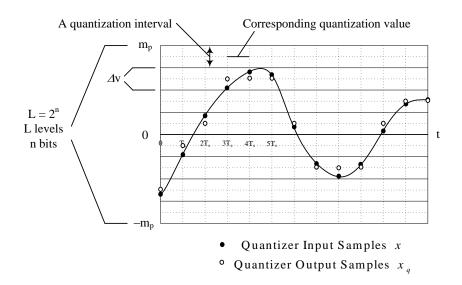
We can define the variable  $\Delta v$  to be the height of the each of the *L* levels of the quantizer as shown above. This gives a value of  $\Delta v$  equal to
