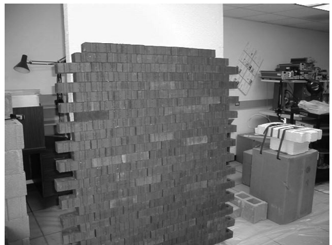
Fig. 2 Illustration of a constructed moving wall for accurate reference measurements
