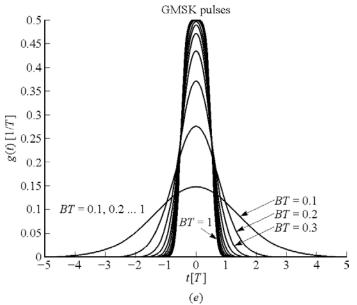
*B, which represents the –3-dB bandwidth* of the Gaussian pulse
