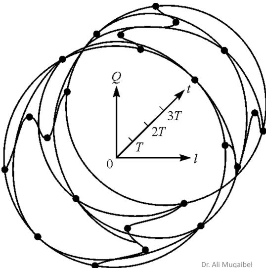
Phase cylinder for binary CPM with  $h = \frac{1}{2}$  and a raised cosine pulse of length 3T. [From Sundberg (1986), © 1986 IEEE.
