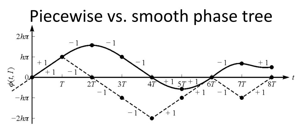
Phase trajectories for binary CPFSK (dashed) and binary, partial response CPM based on raised cosine pulse of length 3*T* (solid). [*From Sundberg (1986), © 1986 IEEE*.]
