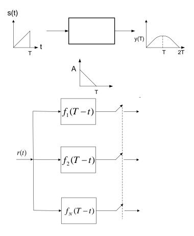
**Property of Matched filter:** If a signal s(t) is corrupted by AWGN, the filter with an impulse response matched to s(t) maximizes the output signal to noise ratio (SNR). Proof :
