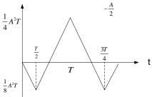
A pair of pulses that are orthogonal to each other over the interval [0,T], are used for two dimensional matched filter
