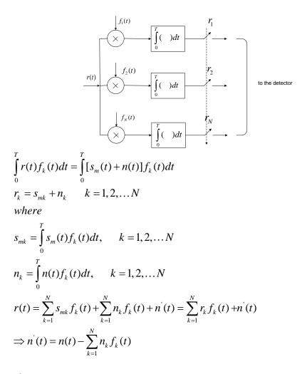
n'(t) is zero mean Gaussian noise process. It is the unrepresented part of noise "inherent". n'(t) is Gaussian because it is the sampled output of a linear filter excited by a Gaussian input.
