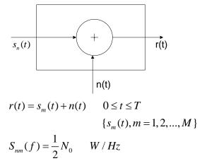
**Objective:** Upon observation of r(t), what is the optimum receiver "design" in terms of probability of making error.
