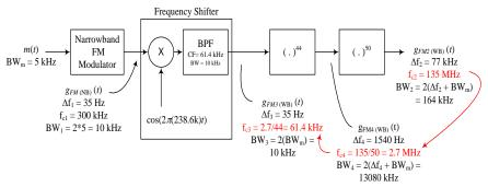
We also can bring the frequency shifter before all the non-linear devices and therefore reduce the frequency of the required oscillator to the minimum value by finding the required carrier frequency at the input of each non-linear device to insure that the carrier frequency of the final output of non-linear devices is the desired final carrier frequency.
