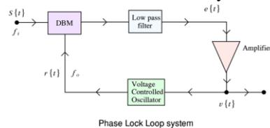
DBM: Double balanced modulator (multiplier)
