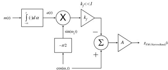
Beta is the modulation index (frequency deviation ratio):  $\beta = \frac{\Delta f}{B}$
