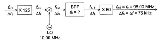
The indirect FM generator (Armstrong) scheme shown, consisting of 5 stages as shown in the figure, stage 1 is the output of the NBFM modulator:
