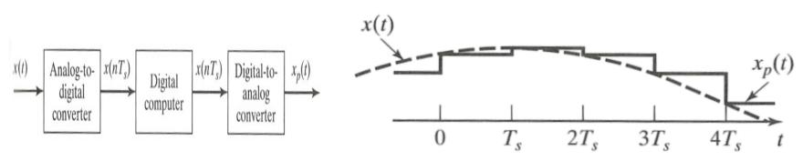
At the output of the sample and hold D2A conversion circuit we can write  $x_p(t) = \dots + x(0)[u(t) - u(t - T_s)] + x(T_s)[u(t - T_s) - u(t - 2T_s)]$   $+ x(2T_s)[u(t - 2T_s) - u(t - 3T_s)]$
