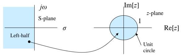
In the s-domain the left-half plane corresponds to  $\sigma < 0$  is mapped to |z| < 1 in the z-plane which is the region inside the unit circle.
