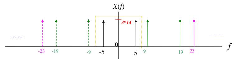
Now, a low-pass filter with cut-off frequency  $= f_s/2 = 7/2 = 7$  Hz. The amplitude of the filter in the low-pass region should be  $1/f_s = 1/14$ . The reconstructed spectrum is exactly like the original signal.
