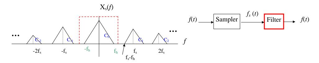
The original signal can be perfectly reconstructed using a low-pass filter with cut-off frequency equals to  $f_s/2$  provided that the original signal was sampled at a frequency above  $2f_h$ .
