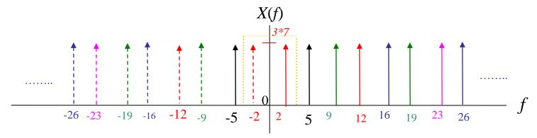
A low-pass filter with cut-off frequency = $f_s/2=7/2=3.5$  Hz is used. The amplitude of the filter in the low-pass region should be  $1/f_s=1/7$ .
