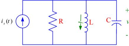
The Laplace transformed circuit is shown in the Figure . (animate)
