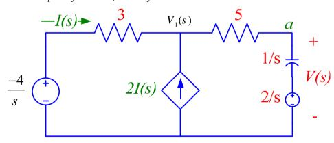
• Note the voltage to be determined is the voltage across the series combination of a 1 F capacitor and a voltage source having a value of v(0)/s=2/s.
