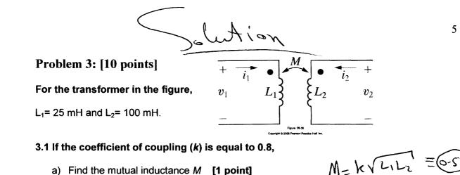
b) Find the turn ratio  $N_2/N_1$ , assuming that the two coils have the same permeance. [1
