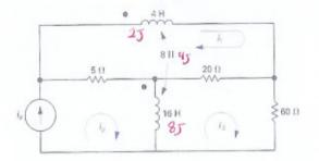
c) Write a set of mesh-current equations that describe the circuit in terms of the currents  $i_1$  and  $i_2$  in the frequency domain, where the source current is known and it has  $\omega = 0.5$  rad/s. (Hint: first represent in the  $j\omega$  domain)
