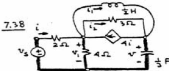
1.  $4\Omega$  resistor chosen for tree
