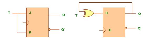
The characteristic equation of the T flip-flop is given by:
