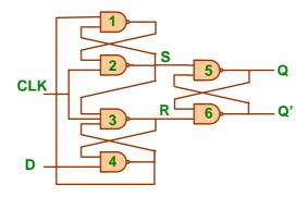
When CLK=0 and D=0, then the outputs of gates 1, 2, 3, and 4 are going to be 0111. If D=1 while CLK=0, then the outputs of these gates are going to be 1110 instead. In both cases, S=R=1, which make Q and Q' are 01 or 10. i.e. one of the two stable states.
