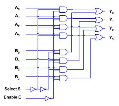
The function table of the quadruple 2-to-1 multiplexer with the enable input will be as follows:
