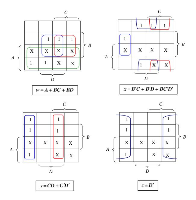
A two level logic diagram can be obtained directly from the logic expressions. Also the logic expressions may be arranged such that:
