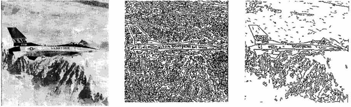
(a) F16; (b) F16, output of LoG; (c) F16, output of the filter.
