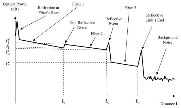
**Figure 2**: Sudden Rise in the Scattered Power when Fiber 2 has a higher Rayleigh Scattering Coefficient than Fiber 1 and Fiber 3.
