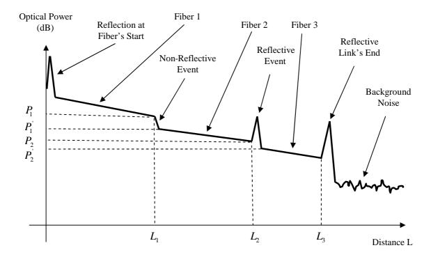
**Figure 1**: An Imaginary OTDR Trace of an Optical Fiber Link Consisting of Three Different Fiber Types Spliced Together. The OTDR Trace Shows the Locations of the Reflective Events, the Non-Reflective Events and the Link's End.
