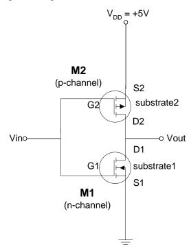
**Figure 3 CMOS Inverter**
