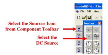
Figure 3: Selection of DC Voltage Source in Multisim
