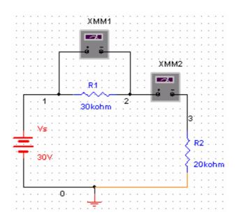
Figure 16: Multimeter connection for current measurement
