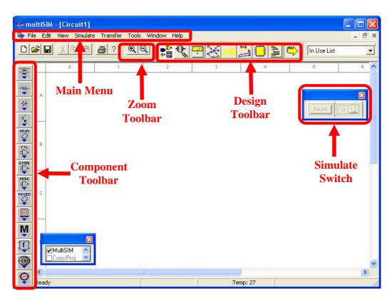
Figure 1: Main Window of Multisim Simulation Software
