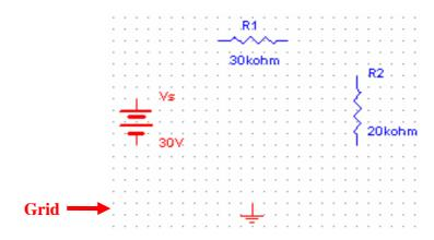
Figure 9: Arranging the Components in proper order
