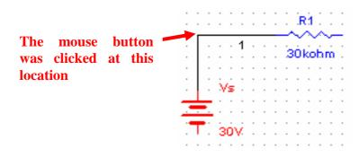
Figure 10: Manual connection of components
