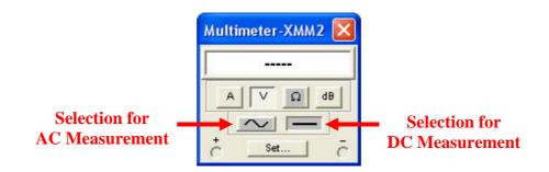
Figure 15: Multimeter properties window
