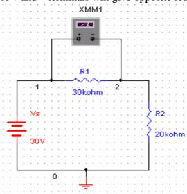
Figure 14: Multimeter connection for voltage measurement
