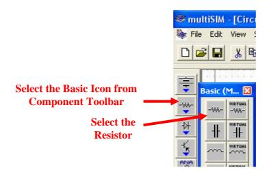
Figure 5: Selection of Resistor in Multisim
