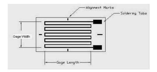
These gages use a grid of fine wire or a constantan metal foil grid encapsulated in a thin resin backing. The gage is glued to the carefully prepared test specimen by a thin layer of epoxy. The epoxy acts as the carrier matrix to transfer the strain in the specimen to the strain gage.
