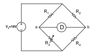
Figure 3: Balanced Bridge Circuit
