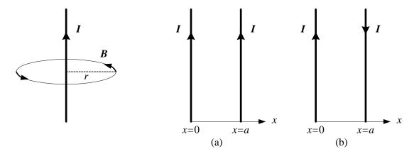
Figure 1: Magnetic field around a straight conductor
