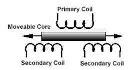
An LVDT is much like any other transformer in that it consists of a primary coil, secondary coils, and a magnetic core. An alternating current, known as the carrier signal, is produced in the primary coil. The changing current in the primary coil produces a varying magnetic field around the core. This magnetic field induces an alternating (AC) voltage in the secondary coils that are in proximity to the core. As with any transformer, the voltage of the induced
