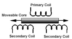
The LVDT is constructed with two secondary coils placed symmetrically on either side of a primary coil contained within the hollow cylindrical shaft. Movement of the magnetic core causes the mutual inductance of each secondary coil to vary relative to the primary, and thus the relative voltage induced from the primary coil to the secondary coil will vary as well.
