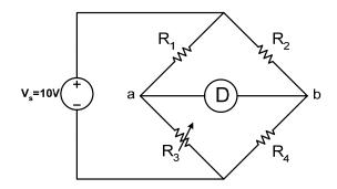
Figure 3: Balanced Bridge Circuit
