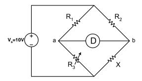
Figure 4: Simplified Wheatstone Bridge Circuit
