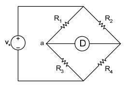
Figure 1: Bridge Circuit.
