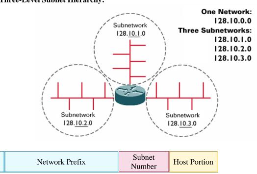
The subnet number now identifies a local <u>segment</u> attached to the <u>router</u>. Because only the network portion of the address is advertised to the Internet, subnetworks are only locally significant. Here's how subnetting works:
