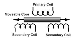
An LVDT is much like any other transformer in that it consists of a primary coil, secondary coils, and a magnetic core. An alternating current, known as the carrier signal, is produced in the primary coil. The changing current in the primary coil produces a varying magnetic field around the core. This magnetic field induces an alternating (AC) voltage in the secondary
