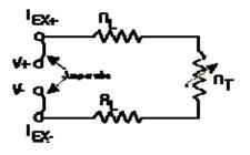
Resistance temperature detectors, or RTDs, are highly accurate temperature sensors. They are also know for their excellent stability characteristics. They are used to measure temperature from 0°C to 450°C, although some can be used up to 800°C. Due to their low resistance values, you must be careful with the RTD lead resistances.
