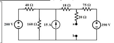
b) If a load resistor  $R_L$  is connected between the terminals a-b as shown in the circuit below, then what is the value of  $R_L$  that will assure a maximum power transfer to it, and what is the maximum power it absorbs. (4 points)
