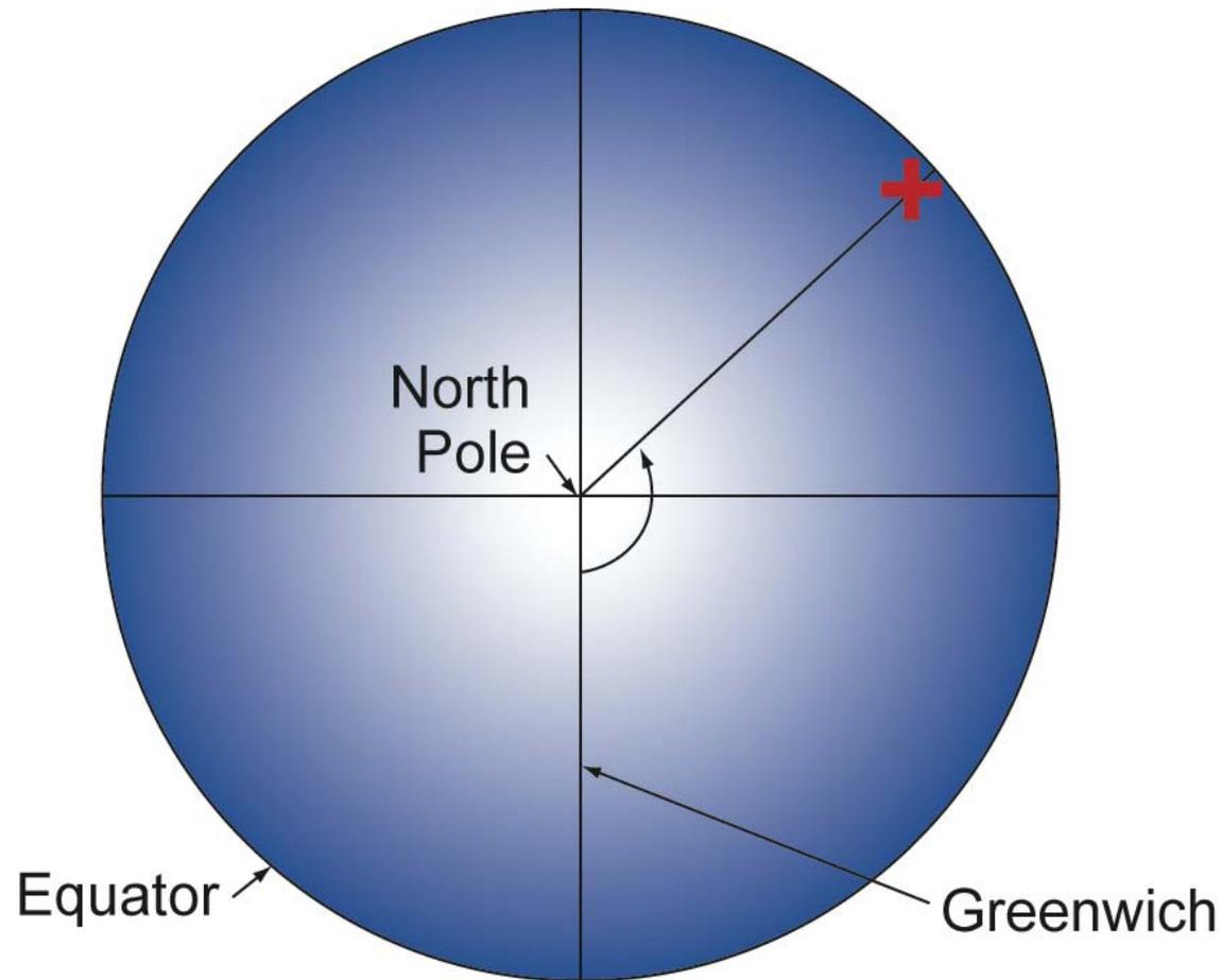
Definition of longitude. The Earth is seen here from above the North Pole, looking along the Axis, with the Equator forming the outer circle. The location of Greenwich defines the Prime Meridian. The longitude of the point at the center of the red cross is determined by drawing a plane through it and the axis, and measuring the angle between this plane and the Prime Meridian.
