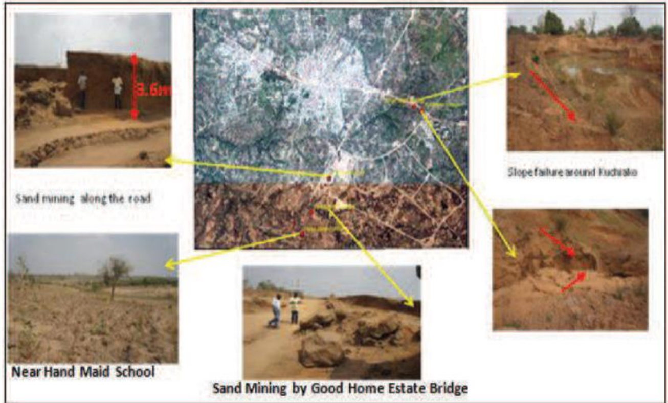
Figure 3: shows sand mining-induced landslide and slope failure scenarios in parts of the study area
