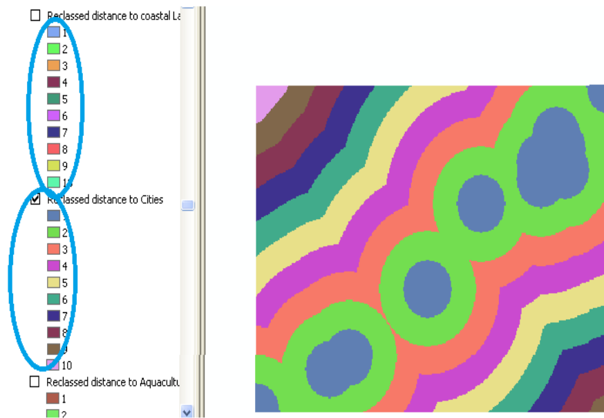
Fig. 15: Data Reclassification; reclassified data layer to represent a populated center (town) (after Balogun et al, 2012)
