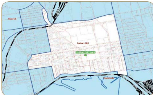
Fig. 1c: This map indicates the addition of cadastre (i.e. erven) and street centre lines. Though the area on the map is not yet definitive, the reference of the map clearly improves with the addition of each layer.
