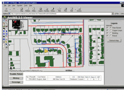
Figure 2 :Typical window of a GIS software of a company in which call center operators can access all the information on a customer and the associated network based on location.
