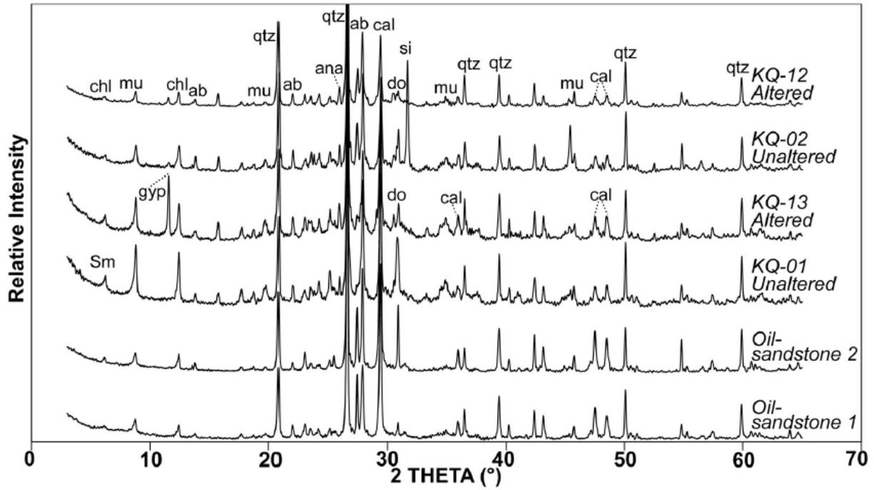
Fig. (10): X-ray diffraction analysis showing mineralogical components of the rock samples collected from the Qiulitage anticline. Ab- albite; ana- analcime; cal-calcite; chl- chlorite; do-dolomite; gyp-gypsum; il- illite; mu-muscovite; qtz-quartz; si- siderite; sm- smectite (Shi et al, 2010).
