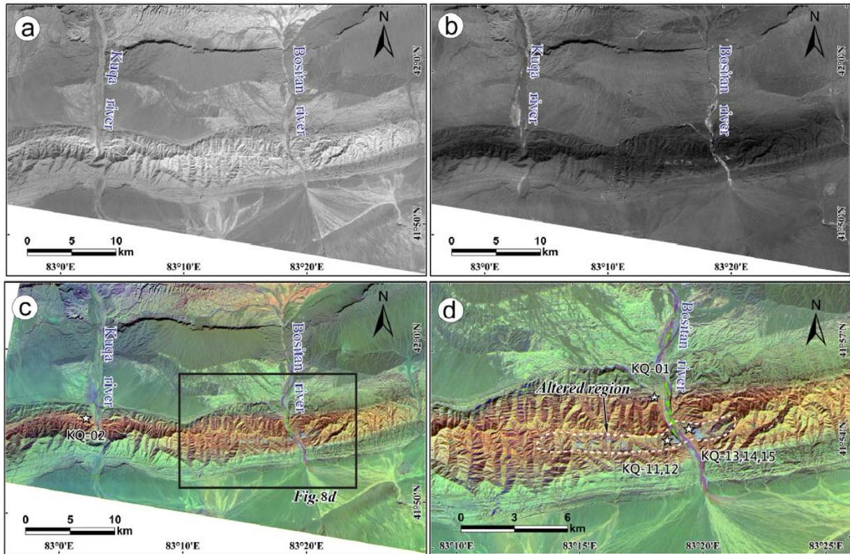
Fig. (8): ASTER images of the study area. (a) Grayscale image of ASTER band ratio 2/1. (b) Grayscale image of ASTER band ratio 4/9. (c) False color composite image of ASTER band ratio 2/1 (R), 3 (G) and 4/9 (B).
