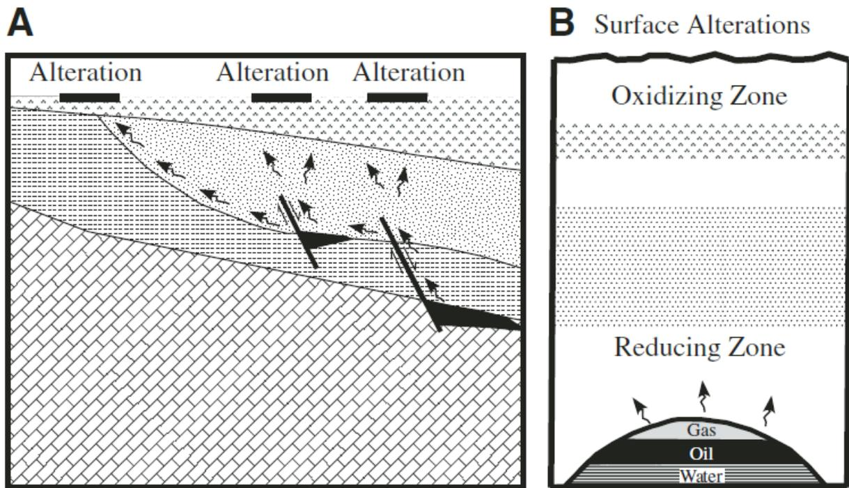
Fig. 1: (A) Processes by which microseeping hydrocarbons migrate from the reservoir to the surface through faults, fractures as well as stratigraphic boundaries (modified from Schumacher, 1999). (B) Generalized model of hydrocarbon induced geochemical alterations of soils and sediments (modified from Schumacher, 1996).
