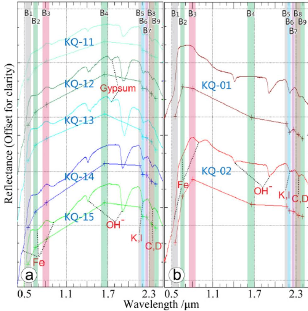
Fig. 7 (a): Reflectance curves of typical altered samples (KQ- 11-15) collected from the Qiulitage anticline. Curves with plus symbols are spectra in ASTER spectral resolution resampled from laboratory spectra. Location of the samples is shown in
