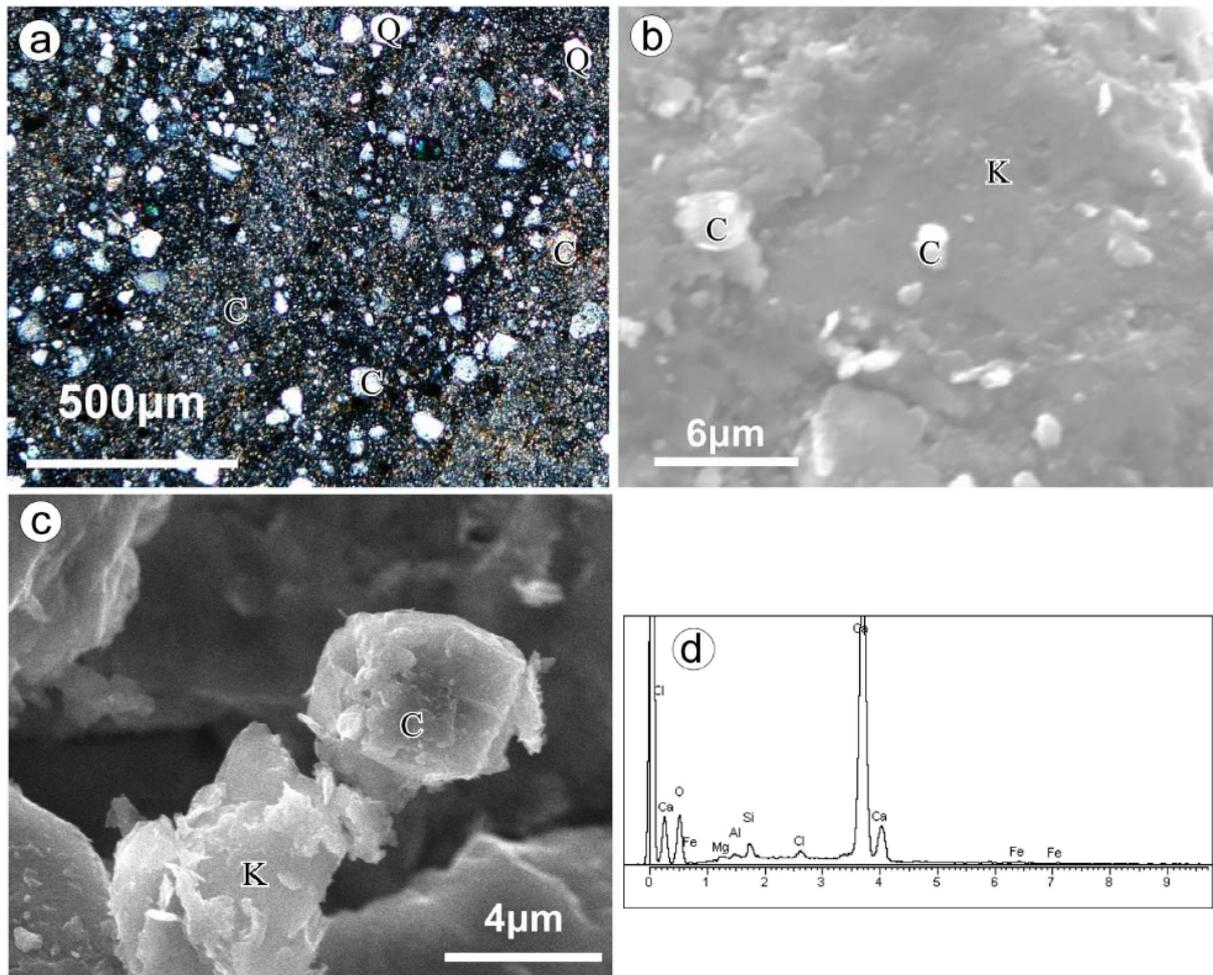
Fig. (9): (a): thin section photo of altered rock sample by orthogonal polarization microscopic study. (2) Scanning electron microscopy (SEM) photo of altered rock sample. Granular calcite mineral particles overlying tabular/platy kaolinite mineral. (3) SEM photo of tabular/platy kaolinite mineral and Granular calcite mineral particles. (4) X-ray energy dispersive spectrum (EDS) of calcite in the altered rock sample. C-Calcite, Q-Quartz, K-kaolinite (Shi et al, 2010).
