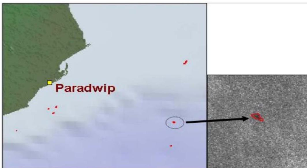
Fig. 3: Hydrocarbon seepages identified in Mahanadi Offshore. The highlighted seepage indicative of Medium degree seepage (Dave, et al., 2011).
