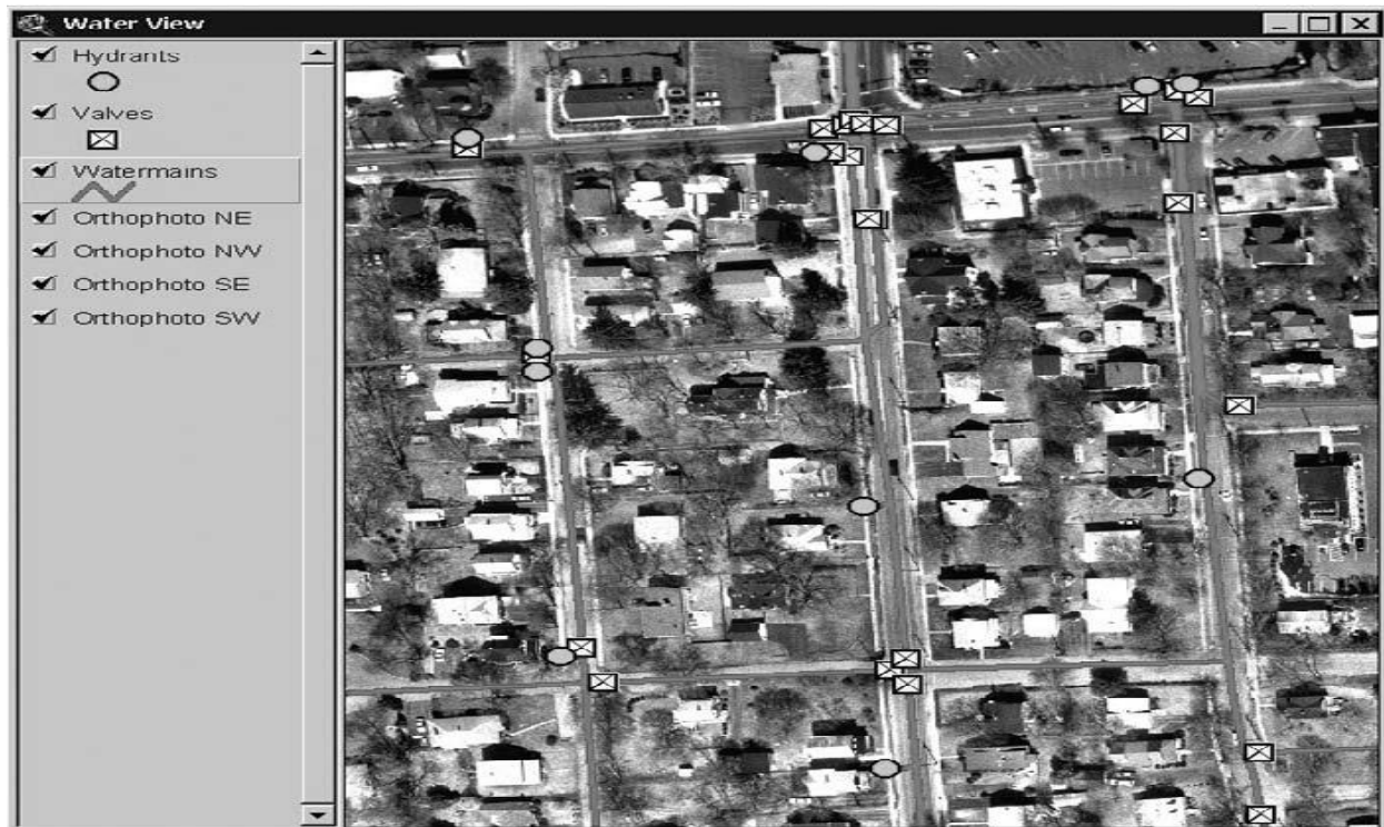
Figure 1. A water distribution system overlaid on a digital orthophoto base map. Source: GIS Applications for Water, Wastewater, and Storm water Systems, Shamsi, 2005.
