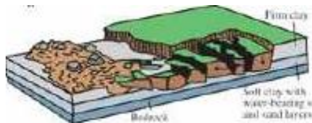
Figure 3: Showing movement of rigid rocks due to lateral extension which underling by softer material at the basal of shear surface (source USGS landslide types and processes)
