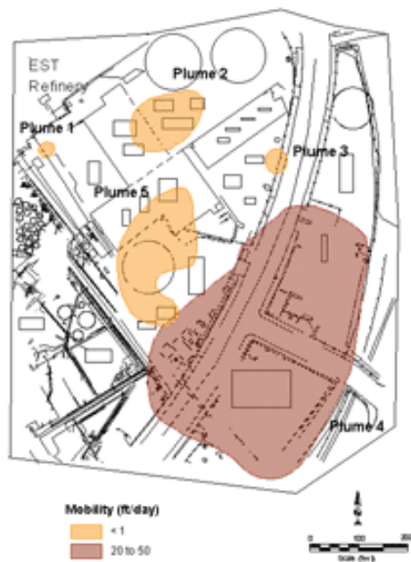
Figure 10: This final map shows mobility across the site. The light brown plume is the only mobile plume among the five plumes.
