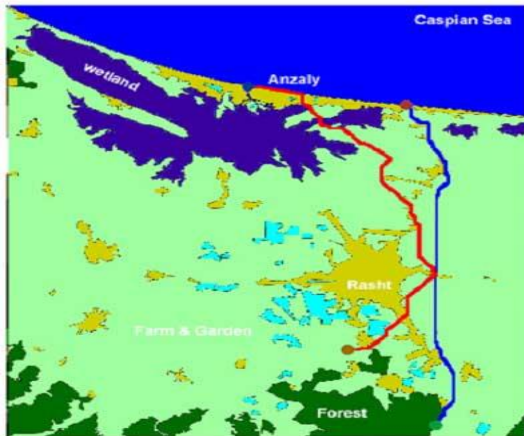
Figure 2. Two Rasht-Anzali alternative railway routes (computed in GIS) overlaid on the Land cover map of the study area
