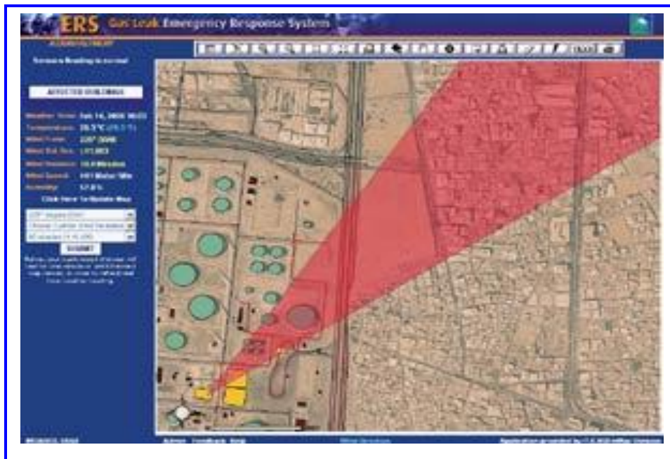
Figure 11. The emergency response system predicts the track of a gas leak. (Source: Emergency Response System-Mapping System, Saudi Aramco).
