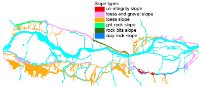
Figure 12c: Seismic stability zonation map of slopes around Lanzhou city (2% probability of exceedance in 50 years) (Wang et.al, 2004).
