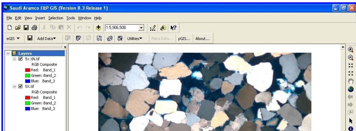
Figure-13: Two illustrations showing how ArcGIS can be used to simulate the microscope view of two images of the same thin section to recognise the minerals from their optical properties.
