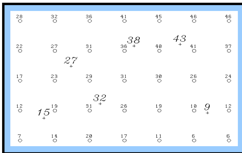
Figure-1 Grid with control points data. (ZmapPlus Mapping (2002), Subsurface Mapping and Non-Default Gridding Techniques. Landmark- Houston USA.)
