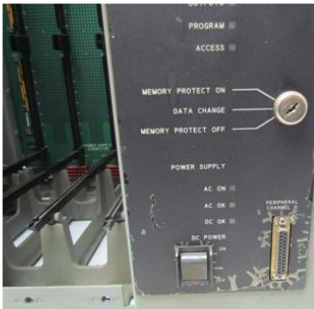
Figure 4 - Typical PLC CPU Security Protection Key Switch
