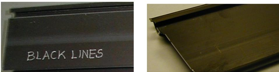
**Figure-7** Black lines show as burnt surfaces on the extrudate due to local high pressures/temperatures.
