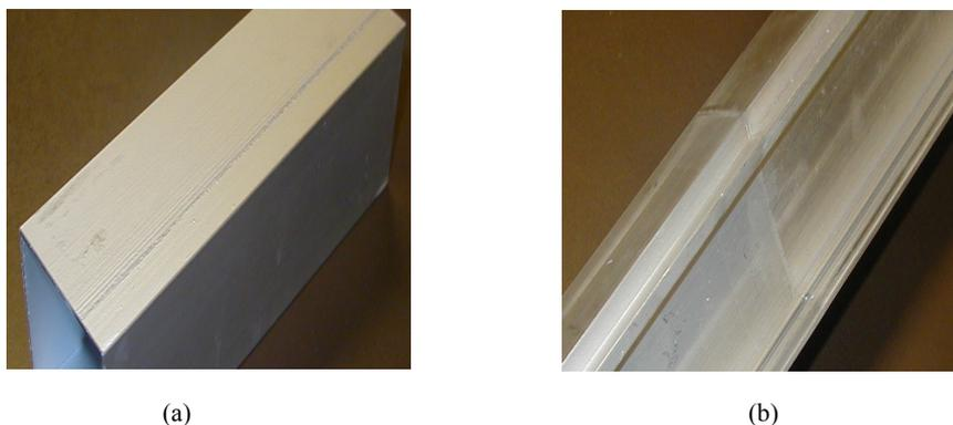
**Figure-5** A die line (a) is a longitudinal depression or protrusion formed on the extruded surface, while a weld line (b) may be due to an imperfect billet-to-billet joint.
