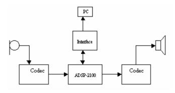
Fig.4.Block diagram of Hardware implementation
