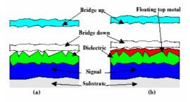
Fig.2: Close-up on the active area showing the parasitic air-gaps as a result of the surface roughness: a) conventional, b) with floating metal
