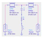
Fig.8: Capacitive shunt switches extraction model
