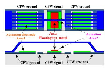
Fig.4: MEMS switch implementing a floating top metal covering the dielectric
