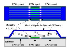
Fig.1: Standard RF-MEMS capacitive shunt switch
