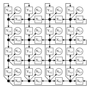
Figure 2a: 2D Torus with 16 nodes, 32 routers, and 16 5-way channels
