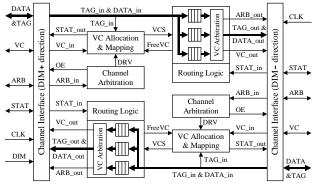
Figure 5: Internal Architecture of a Router
