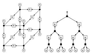
Figure 3: 3D cube with 4-way channels and a tree with 3-way channels
