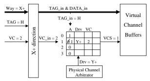
Figure 7: Allocating a virtual channel for a header flit
