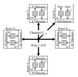
Figure 2b: Structure of a Multiway Channel
