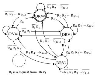
Figure 6a: FSM of the Channel Arbitrator
