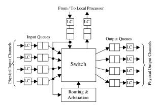
Figure 1: Generic wormhole router used in k-ary 2-cube networks
