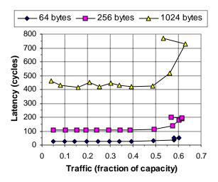
Figure 8c: Latency versus traffic under different message lengths
